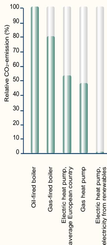
Relative CO<sub>2</sub> emission of heating devices.
