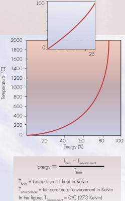
temperature at which it flows. Indeed the exergy content of heat varies in temperature as shown by the curve and the formula on the left.
