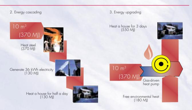
Figure 1: By developing energy systems with energy cascading and energy upgrading, much better use is made of energy resources than with the traditional approach.
